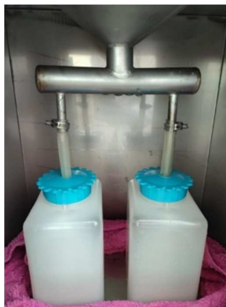
Figure 8. Rainwater sample bottles inside the device
